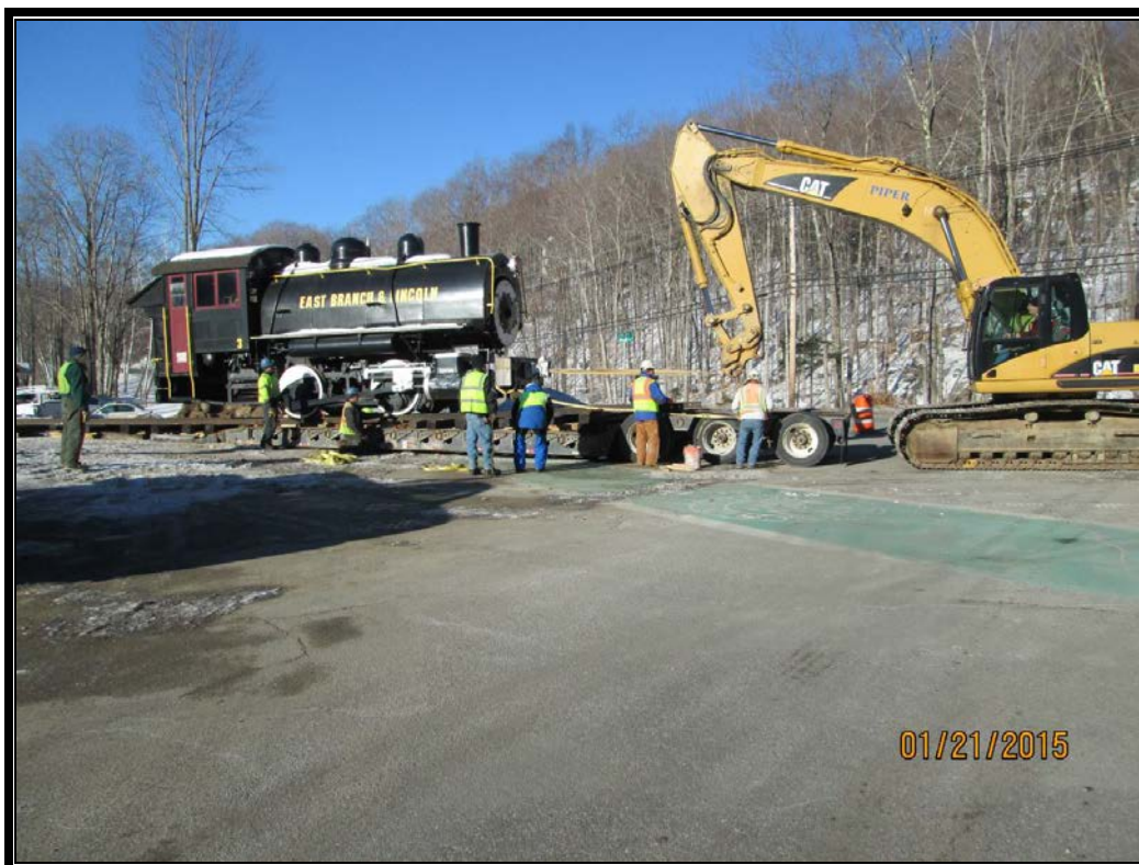
Photo 5: Excavator pulling locomotive onto modified trailer.
